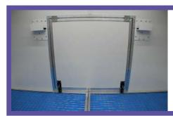
An emergency "quick release" exit panel is fitted as standard in the rear wall of the spray room to comply with **HSE recommendations**.
