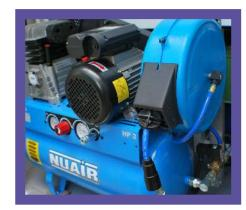
A 3HP compressor and retractable air reel are fitted as standard.
