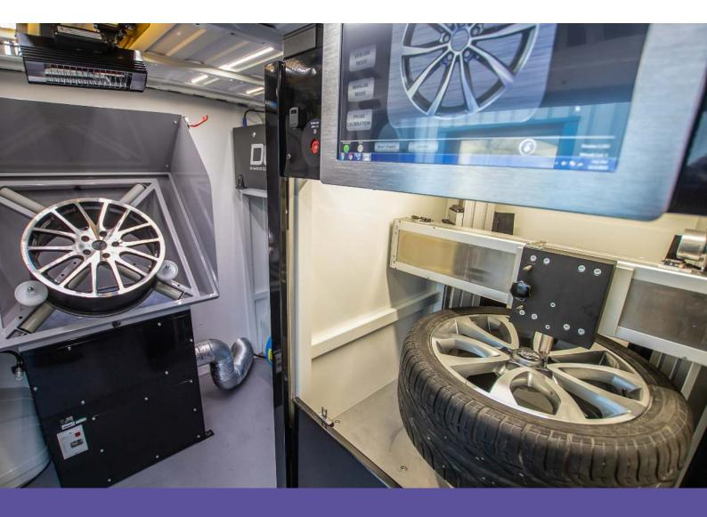
The **SMARTvan® Diamond** is the first mobile facility to feature a full **CNC Lathe** for the repair of Diamond Cut alloy wheels.
