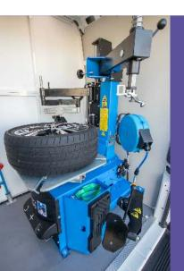
We supply a full size semi automatic tyre changer for the removal and refitting of tyres.
