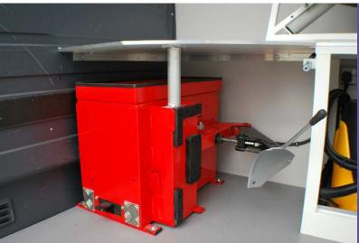
For breaking the tyre bead, we supply and install a **full size tyre machine** base.
