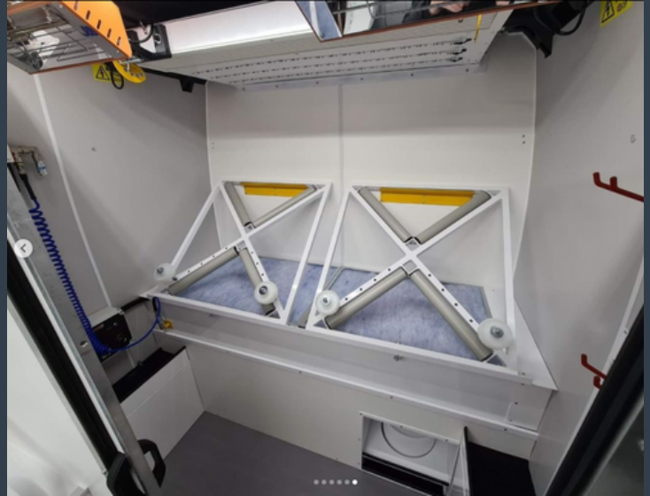
Fully segregated spray room with integrated infra red heaters
